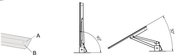
The angle of inclination can be programmed; FOLD! display will then always move to the saved position:
