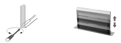
Each FOLD! series monitor is equipped with DIRECT AXLE ACCESS (DAA), a useful feature for installation and maintenance. This allows you to manually extend and retract the monitor, i.e. without power. Access is located on the lower right and left sides of the housing. You need a slotted screwdriver or a cordless screwdriver to operate it.
