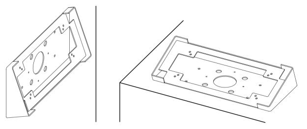
**2.** Mark holes for mounting and inwall charging cable.
