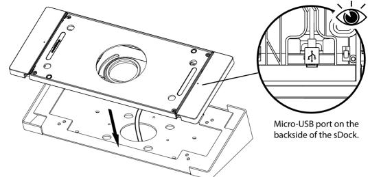
6. Use included screws to fasten the sDock on your Triangle by pressing down the frame.
